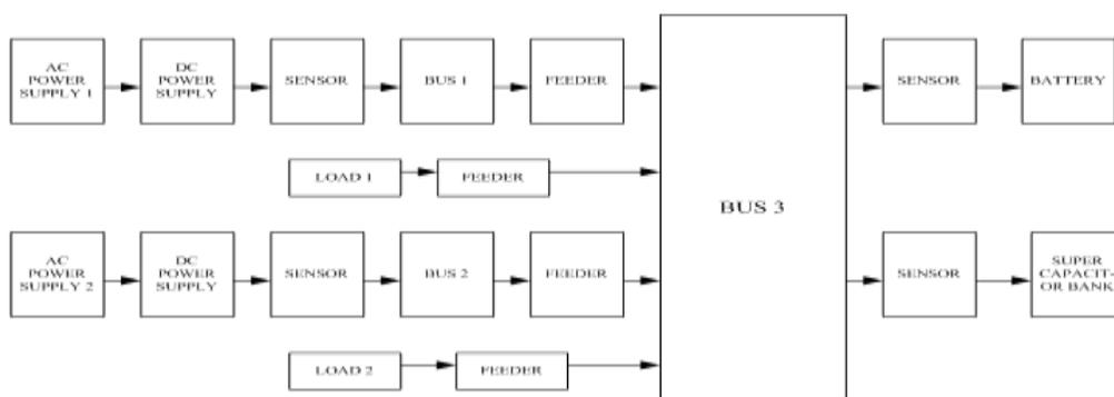
Fig1. Proposed schematic model under study of dc micro-grid.
