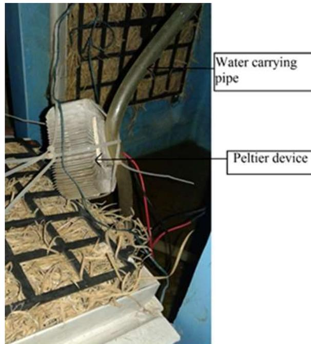
**Figure 4: Peltier device**
