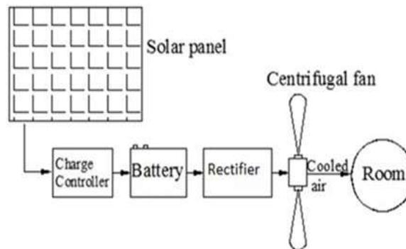
Figure 2: Solar energy conversion process
