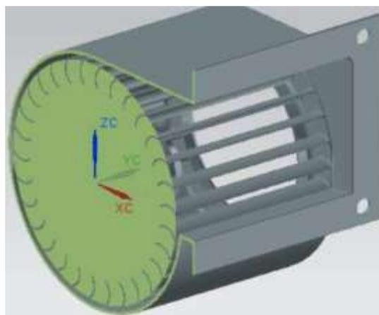
Figure 3: Section view of the fan
