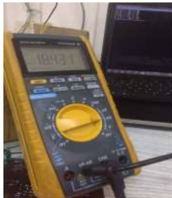
Fig.6 Ammeter Reading while Receiving Data
