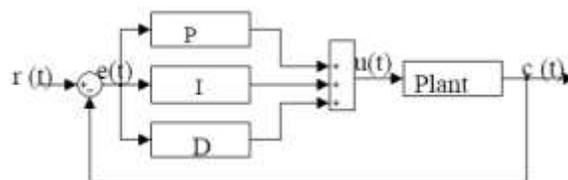
**Fig.1 The conventional PID control system**
