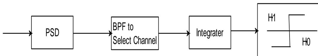
Figure 3: Energy detector block diagram [11]
