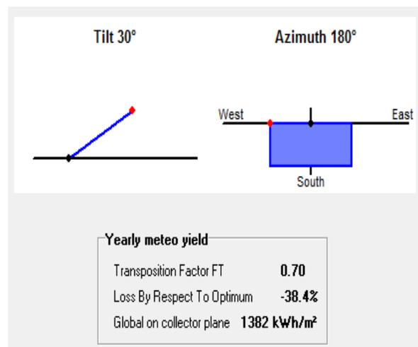
**Fig. 2. Orientation of PV array**
