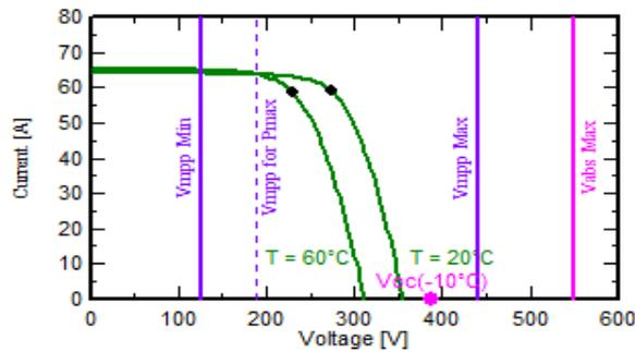
**Fig. 3. Array and inverter voltage sizing**
