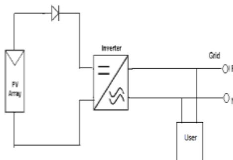
**Figure 1. Grid Connected PV system**
