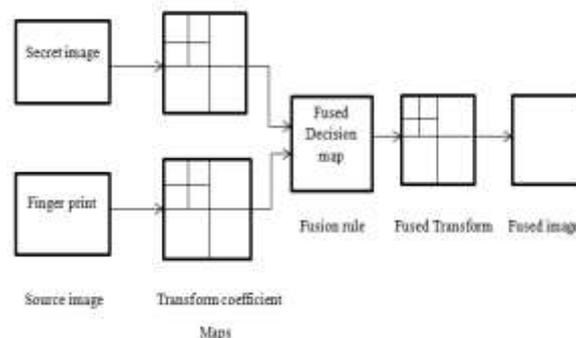
Fig.2 Transform based image fusion
