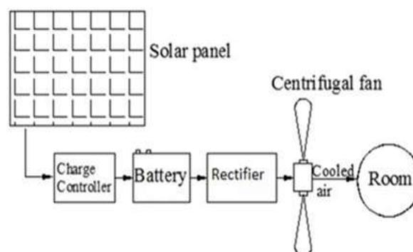
Figure 2: Solar energy conversion process
