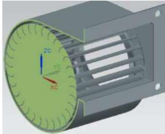
**Figure 3: Section view of the fan**
