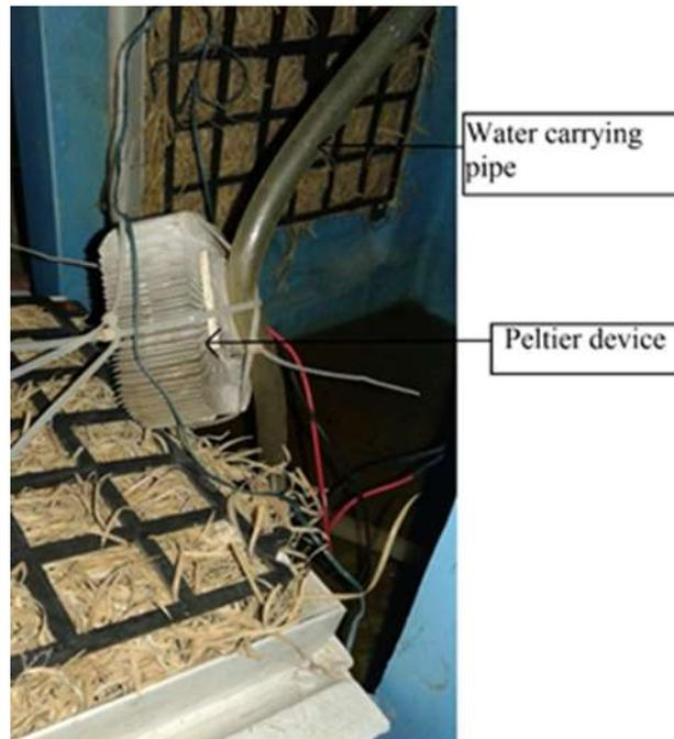
Figure 4: Peltier device
