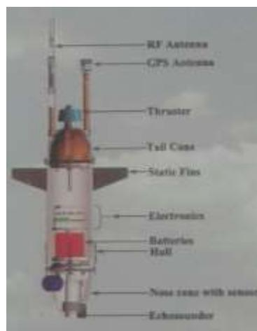
**Fig1: Autonomous Vertical Profiler (AVP)**
