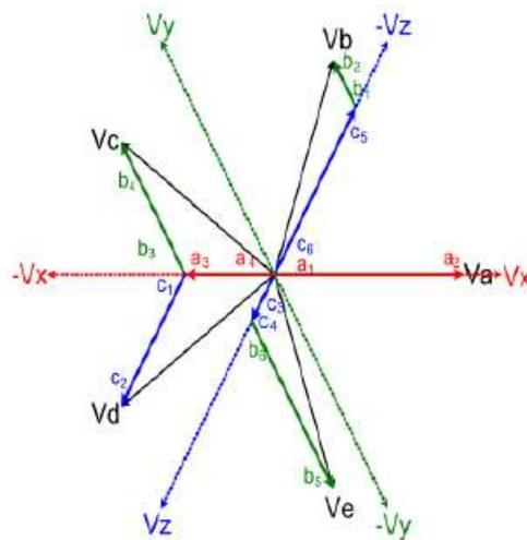
Figure 4-Phasor Diagram for Input Star-Output Star Connection
