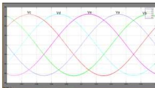
Figure 7-Output Voltages  $V_a=V_b=V_c=V_d=V_e=325V$ (pk-pk)
