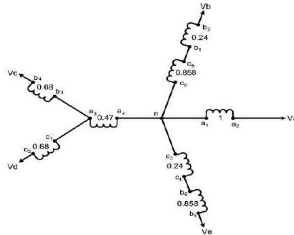
Figure 3-Transformer secondary winding connection
