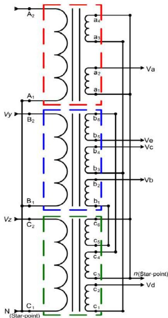
Figure 2-Transformer Winding arrangement
