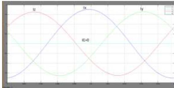
**Figure 12-Three Phase Input currents**
