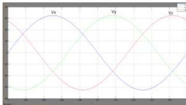
Figure 6-Input Voltages  $V_x=V_y=V_z=325V$ (pk-pk)
