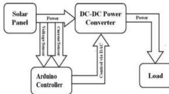
Figure 2. Block Diagram of MPPT System
