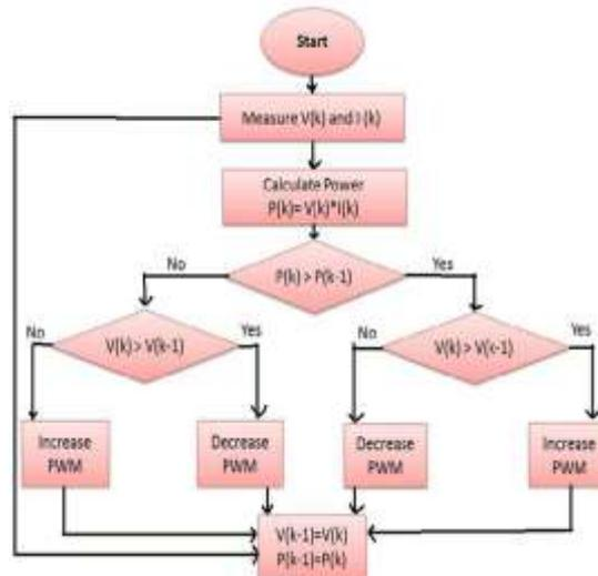
Figure 5. Perturb & Observed Alogrithm
