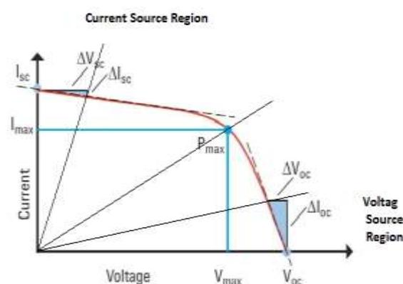
**Figure 1. Voltage Current & Power Voltage Characteristics**
