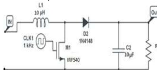
Figure 4. DC-DC Converter
