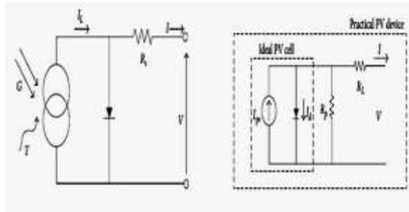
Figure 3. Equivalent Circuit of PV Cell
