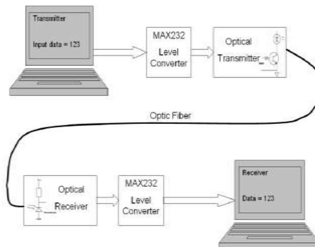
**Fig: Block Diagram of PC to PC Communication Using Optical Fiber Cable**
