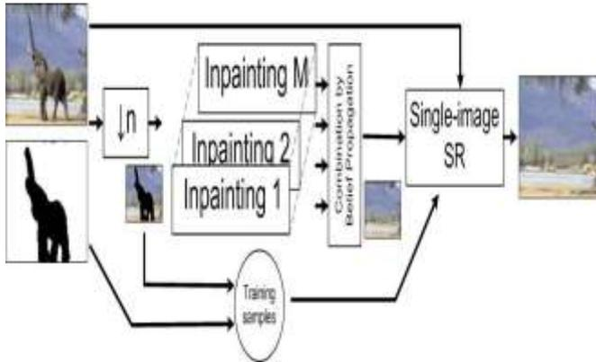
Fig. 1. The framework of the SR method.
