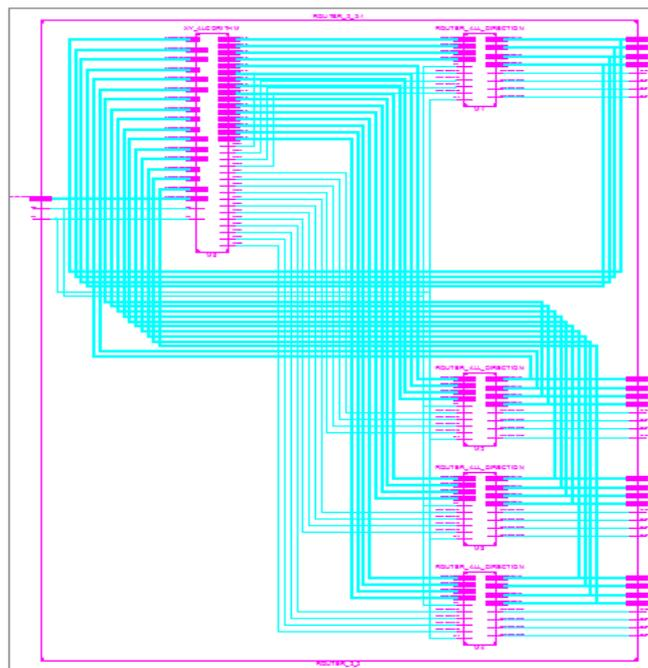
Figure 5: RTL Schematic of 2x2 Mesh topology using XY routing algorithm
