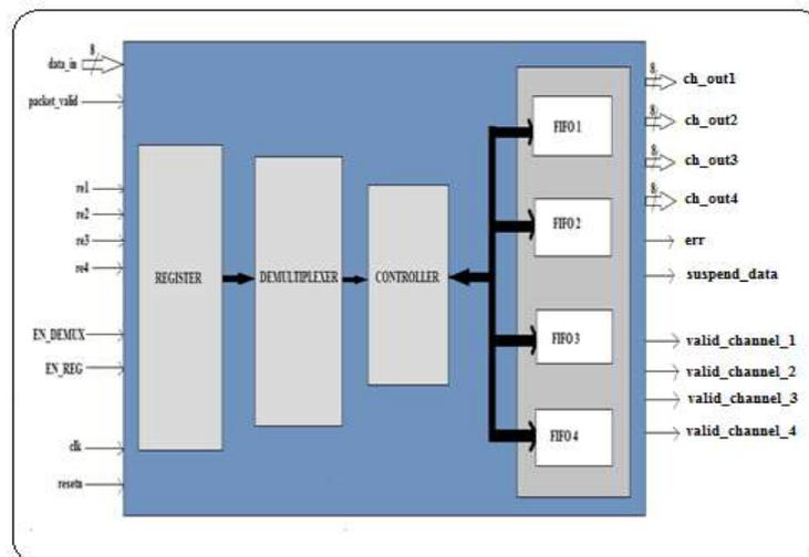
**Figure 3: Internal Structure of Router Block**
