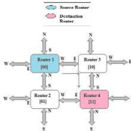
**Figure 2: 2X2 Mesh Topology with Router Address showing Routing Path**
