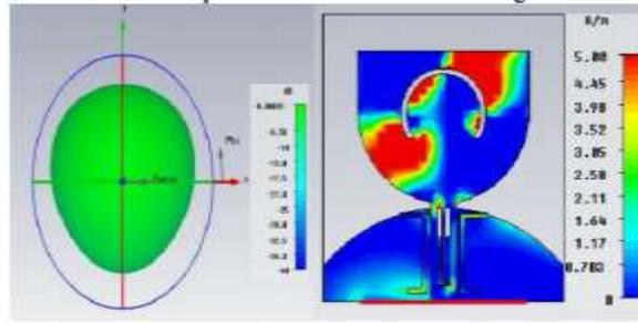
Figure 9. Radiation pattern and Surface current distribution at 4.7GHz
