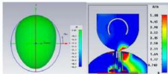
Figure 11. Radiation pattern and Surface current distribution at 7.5GHz
