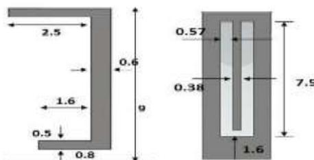
Figure 3. C-shape slit and the U-slot
