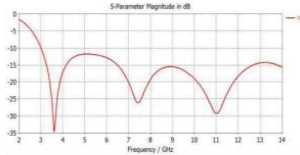
Figure 2 Return loss vs frequency curve of proposed antenna
