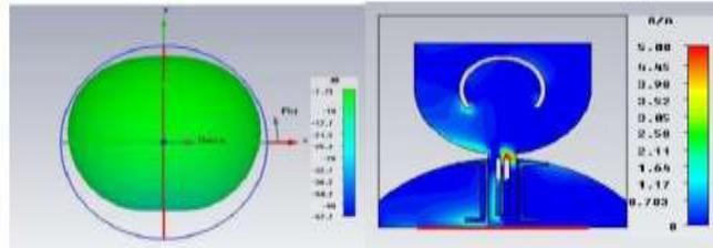
Figure 10. Radiation pattern and Surface current distribution at 5.6GHz
