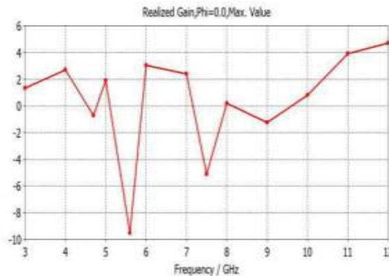
Figure 12. Realized Gain vs Frequency plot
