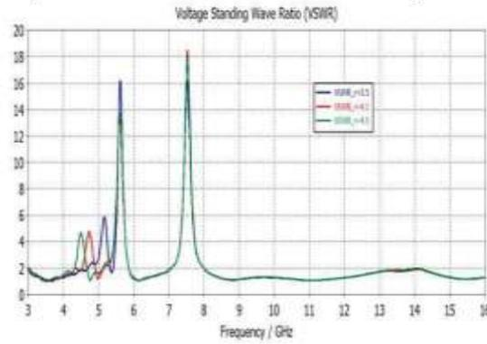
Figure 6. vswrvs frequency curve for different radius  $r$  of annular ring.
