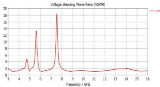
Figure 4. vswr frequency curve of Proposed Antenna.
