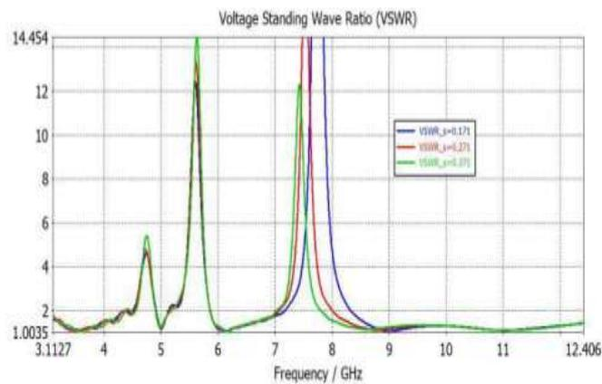
Figure 5. vswr frequency curve for different values of  $s$  spacing between slits and feed line
