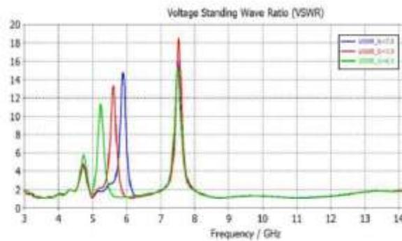
Figure 7. vswrvs frequency curve for different length  $L1$  of Ushape notch.
