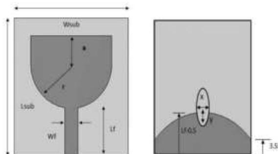
Figure 1. Front and back view of UWB antenna
