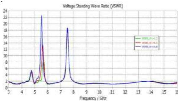
Figure 8. vswrvs frequency curve for different Width  $w1$  of Ushape notch.
