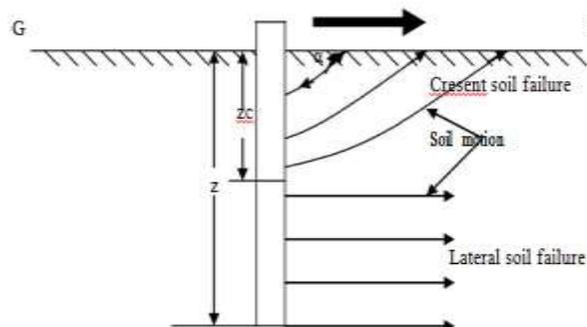
**Fig. 3: Soil movement for a very narrow cutting tool**
