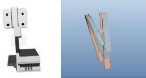
**Fig. 4: Clamping Device and set of the Tyne**
