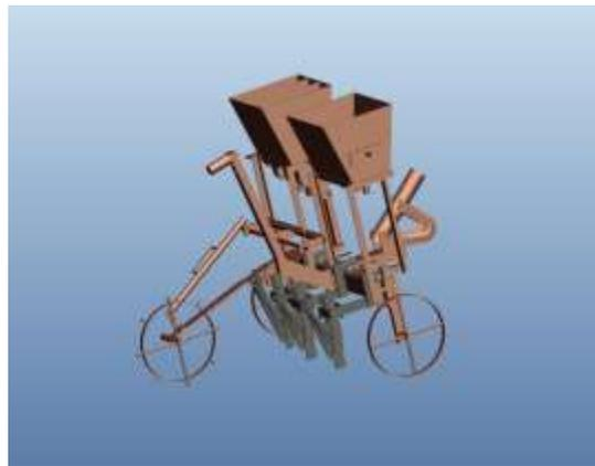
**Fig. 1: Pro-E 3D view of Assembled Model**
