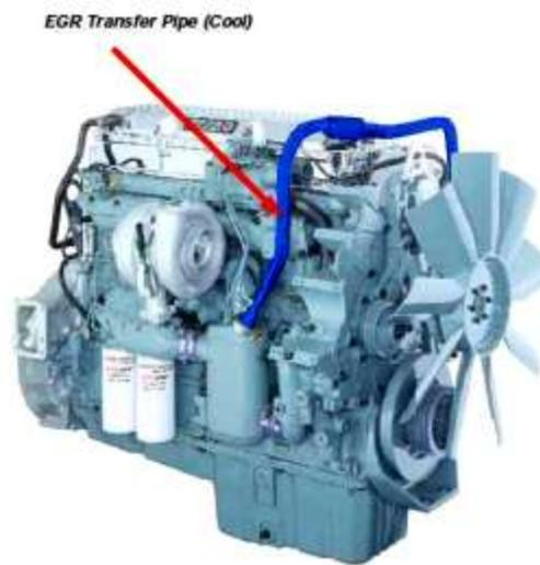
The cooled exhaust gases then flow through the EGR transfer pipe into the intake manifold.
