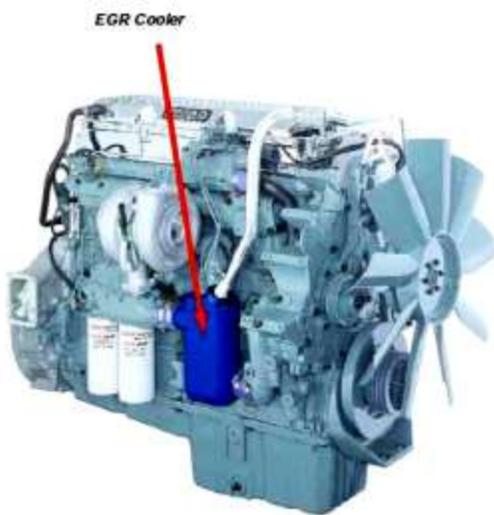
The exhaust gases are cooled by water from the truck cooling system.
