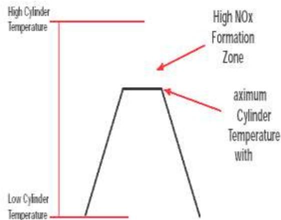
**Fig2.NoX Reduction By Lowering The Temperature.**
