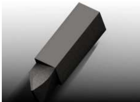
Fig.2: - Single point cutting tool in CATIA.
