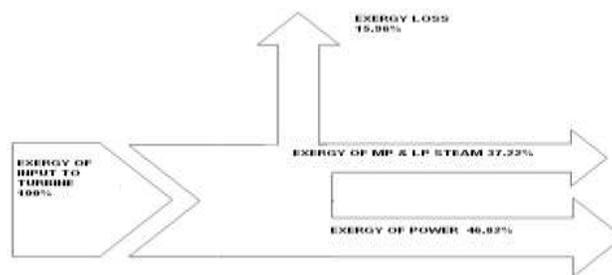
**Figure 3: Sankey diagram for exergy flow through steam turbine at 100% MCR**
