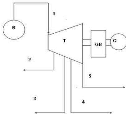
**Fig 2 Process Flow Diagram of Extraction Condensing Steam Turbine**
