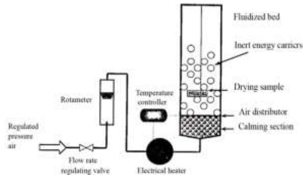
**Fig. 2: Schematic diagram of Fluidized Bed Drying**
