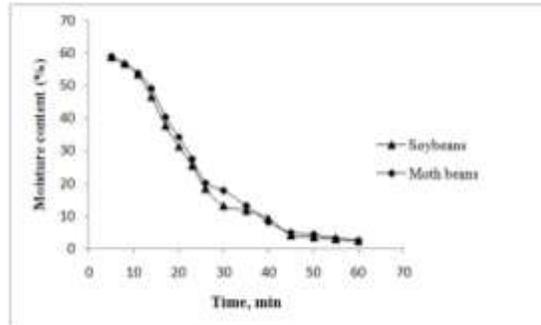
Fig.5: Comparative Drying curve
