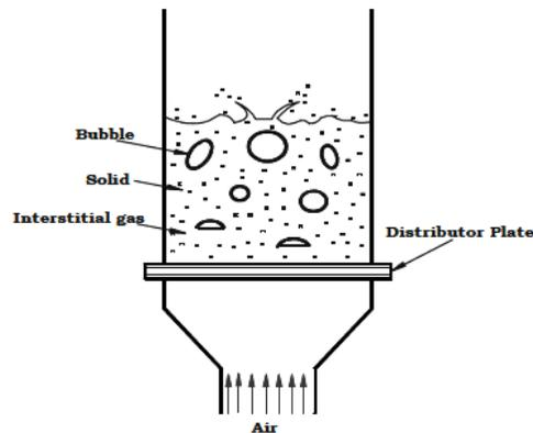
**Fig.1: Bubbling Fluidization processes**
