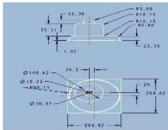
**Fig: 1 Part drawing of protection cap**
