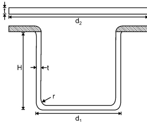
Total surface area of blank = total surface area of component
