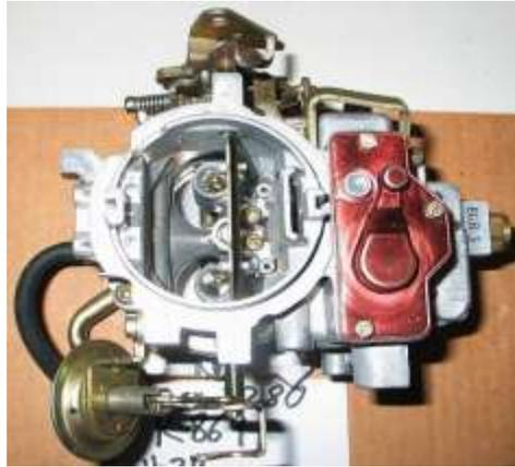
Figure 3: Multi Barrel Carburetor
