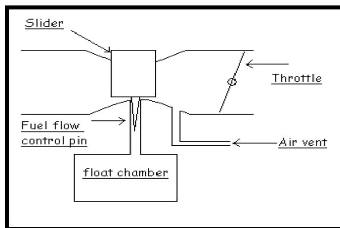
Figure 4: Position of Air Vent
