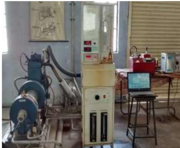
Fig. 2: Kirloskar make Single Cylinder Four Stroke Diesel Engine
