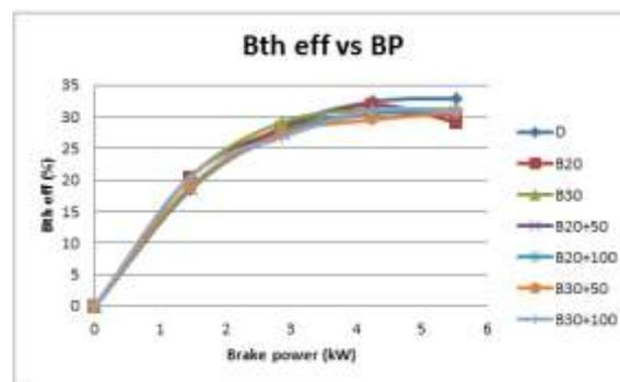
Fig 3.B: Brake Thermal Efficiency Vs Brake Power
