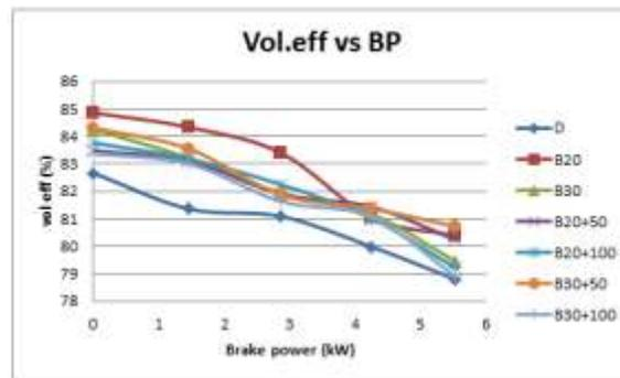
Fig 3.C: Volumetric Eff. Vs Brake Power
