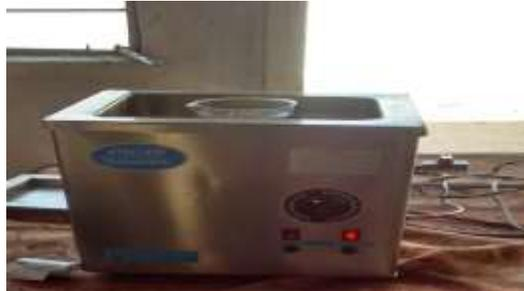
**Fig 1.2: Nano fluid preparation, Ultrasonicator**
