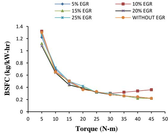
Fig 3.4: BSFC (kg/kW-hr) Vs Torque(N-m)
