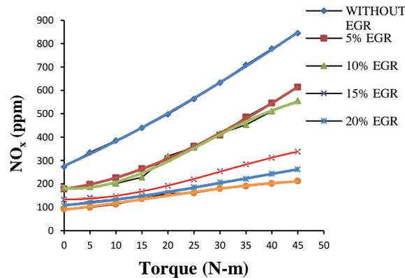
Fig. 3.1 : NO<sub>x</sub> (ppm) Vs Torque (N-m)
