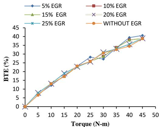
Fig 3.5 BTE (%) Vs Torque (N-m)
