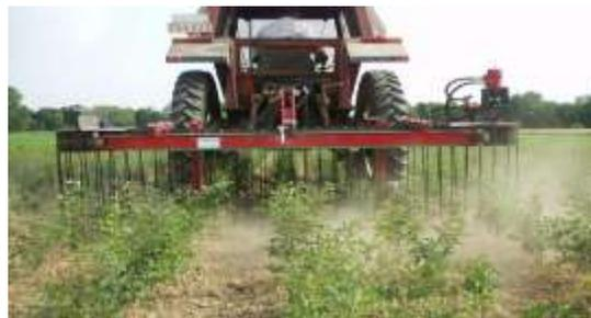
**Figure 5: Mechanically tilling around plants**
