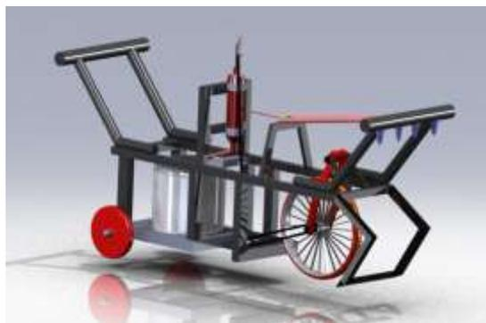
**Fig. 11 CAD model of agricultural pesticide sprayer**
