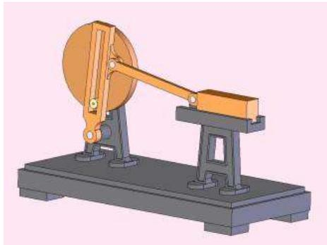
**Figure 9: Crank (mechanism)**
