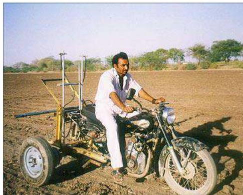
**Figure 3: Motorcycle driven spraying**
