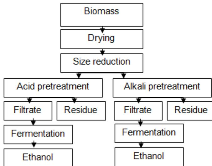
**Fig 1 schematic diagram of biomass pretreatment**
