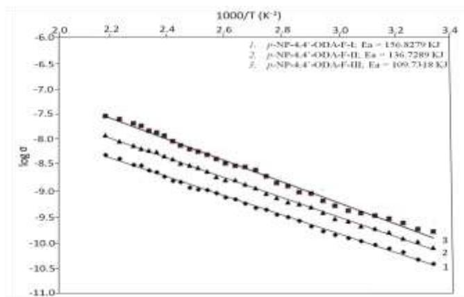
**Figure (1). Electrical conductivity plots of *p*-NP-4,4'- ODA- F copolymer resins.**
