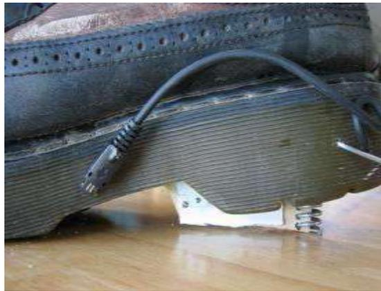
**Fig 5: footwear embedded harvester**
