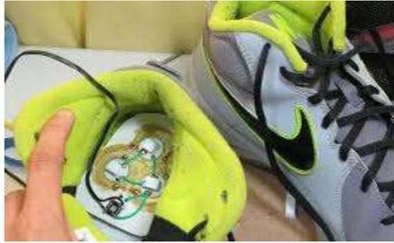
**Fig 6: piezoelectric shoe**
