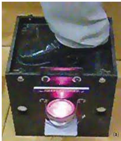
**Fig 3: Footstep electric converter device**
