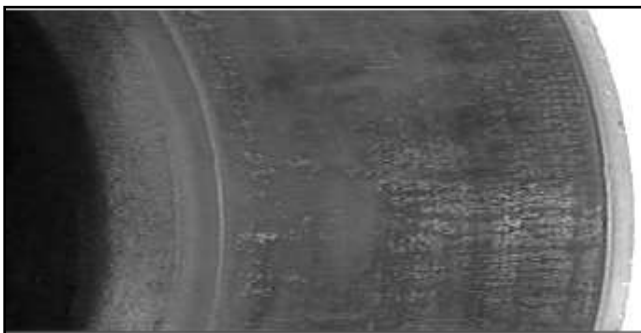
Figure 1.3 Deep Wear on One Side of the Drum Only
