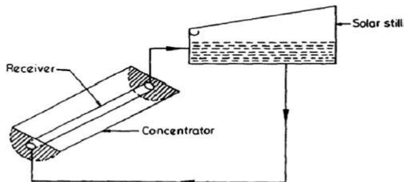
**Fig. Concentrator assisted solar still**
