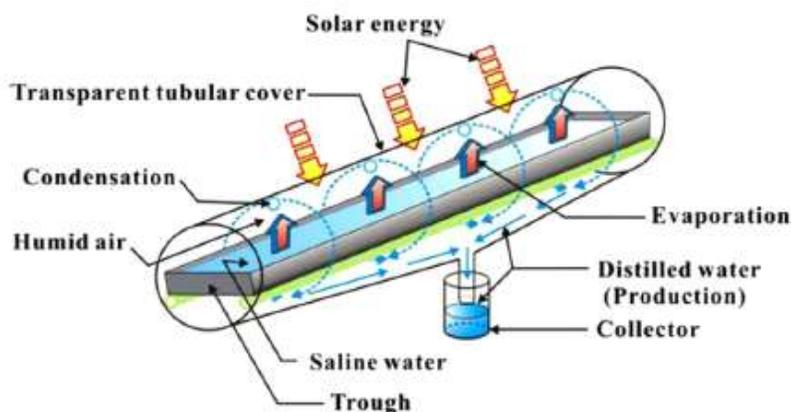
**Fig. Mechanism of pure water production from tubular solar still**
