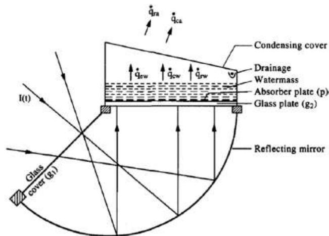
Fig. Inverted absorber solar still
