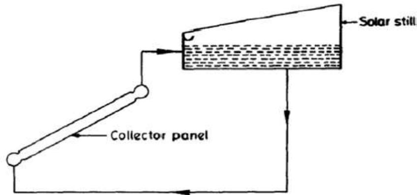
**Fig. Flat plate collector assisted solar still**
