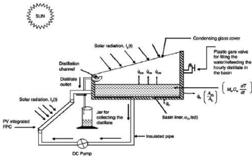
Fig. Hybrid PV/T integrated solar still
