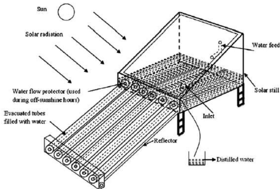
**Fig. Solar still coupled with evacuated tube collector**
