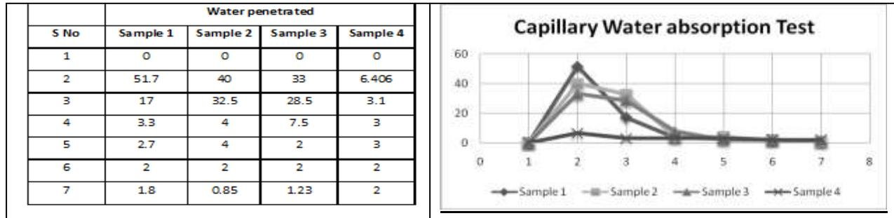
Figure (6): Capillary water Absorption results and Analysis.
