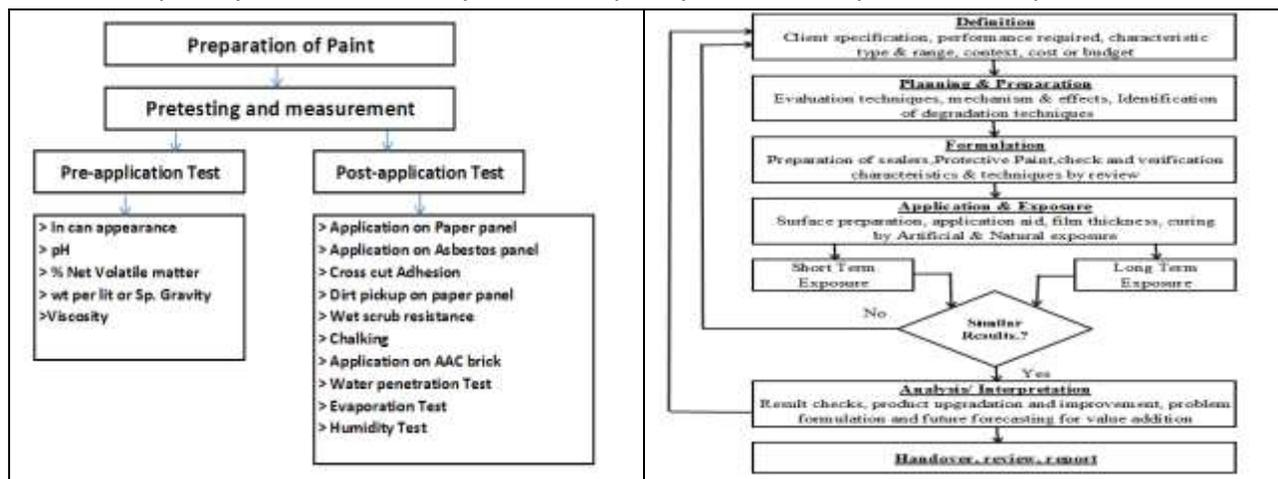
Figure [5]: Paint applications Methodology for Protective coating and Performance Testing.
