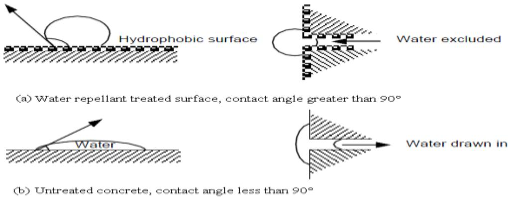
Figure (4): The principle of water repellency.
