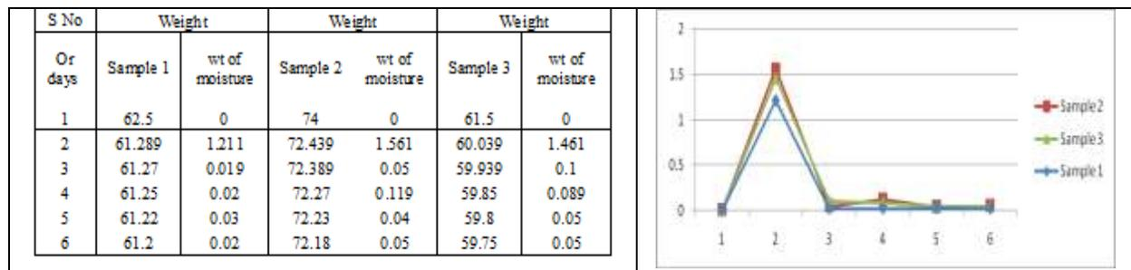
Figure (7) :- Water Evaporation Test Table & Analysis.
