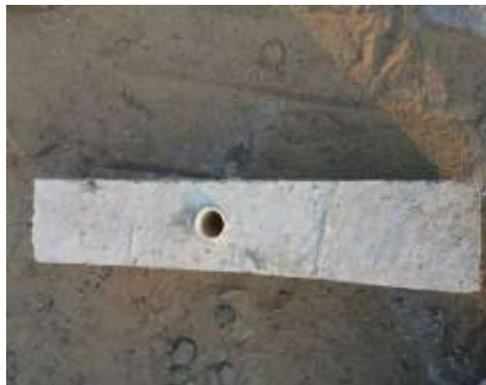
**Figure 3: RCC beam Sample with web opening**
