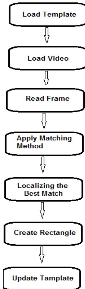
**Fig.1 Algorithm flow diagram:**
