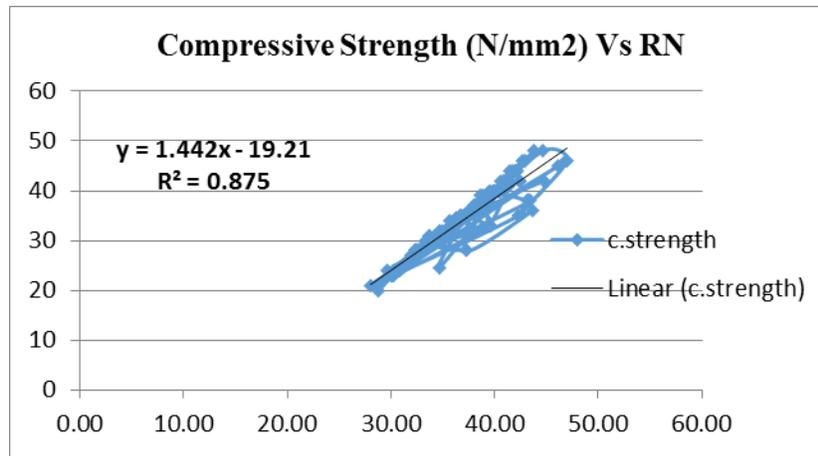
Fig 3 compressive strength Vs Rebound number
