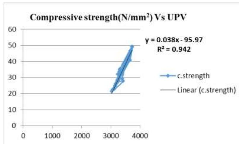
Fig 4 compressive strength Vs UPV
