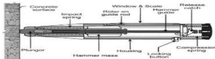
**Fig 1 Rebound Hammer with Various Parts**
