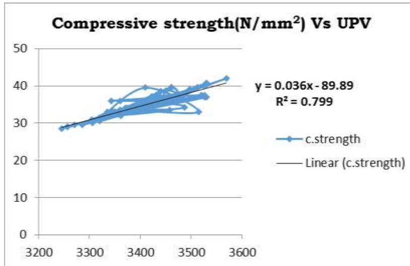
Fig 6 Compressive strength Vs UPV
