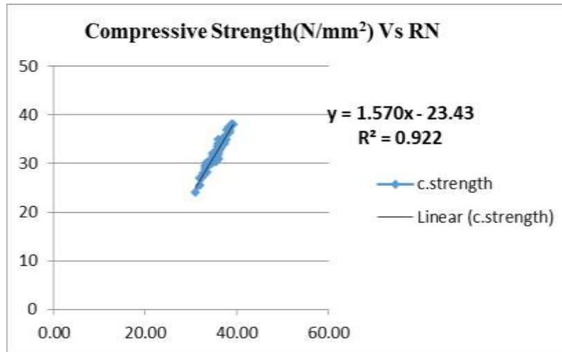
Fig 5 Compressive strength Vs Rebound number
