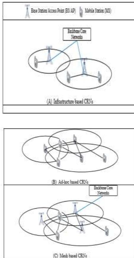
Figure 3. Architecture of Cognitive Radio Networks
