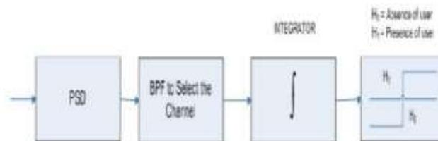
**Figure 5: Energy detector diagram**
