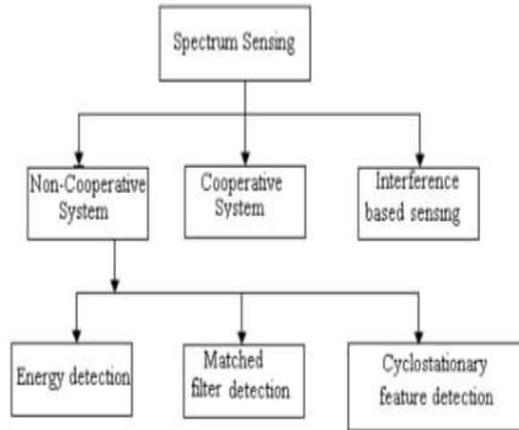
**Figure 4: Classification of spectrum sensing techniques**
