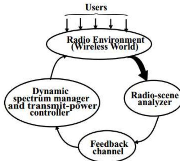
Figure 2. Basic signal-processing cycle, as seen by a single user (transceiver).
