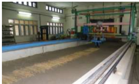
Fig. 2 Experimental set-up of straw cutting mechanism
