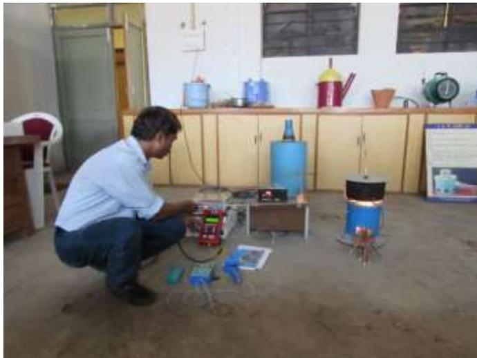
**Fig. 2 Complete set up for evaluation of thermo-efficient cook stove**
