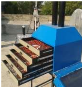
Fig. 2 Tomato slices loaded in solar cabinet dryer
