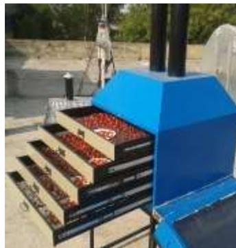
Fig. 2 Tomato slices loaded in solar cabinet dryer
