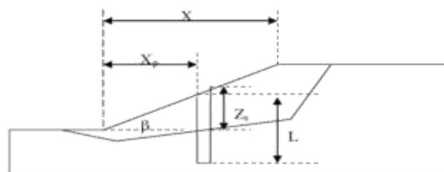
Figure 1: A profile of pile stabilized slope
