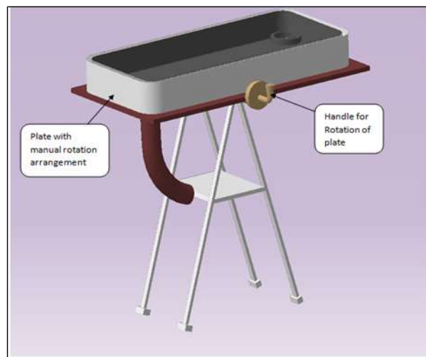
Fig 4: Prototype for Improved solar air preheater system
