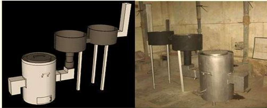
**Fig 2: Schematic diagram of cross draft biomass gasifier cook stove**
