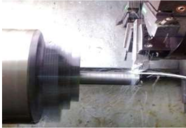
Fig. No. 4 Machining of EN 19 alloy steel
