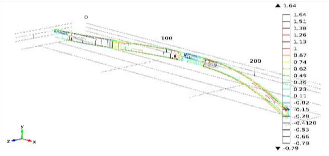
Figure 3 (a): Graph showing Principal stress plot on the microcantilever
