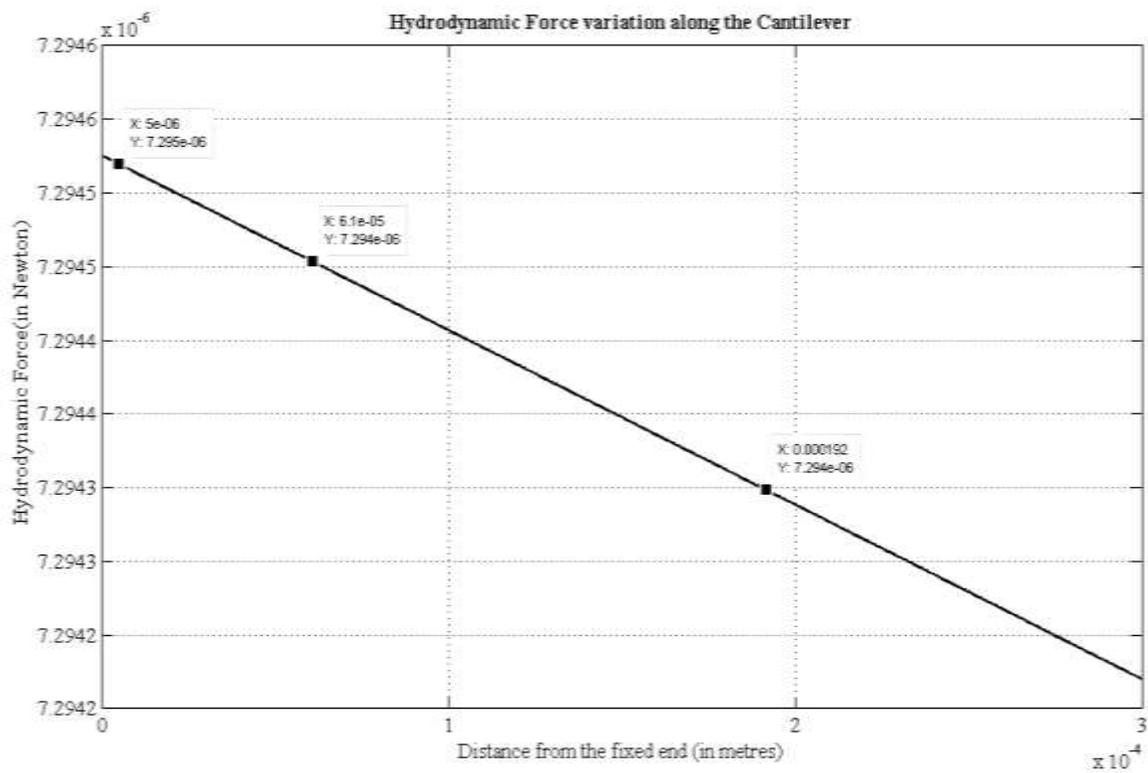
**Figure 2: Graph showing variation in Hydrodynamic force along length of cantilever**
