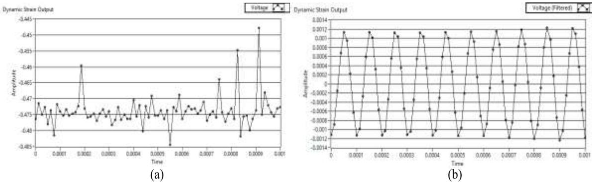
Figure 9: Dynamic strain output at time instant t3 (a) Unfiltered (b) Filtered
