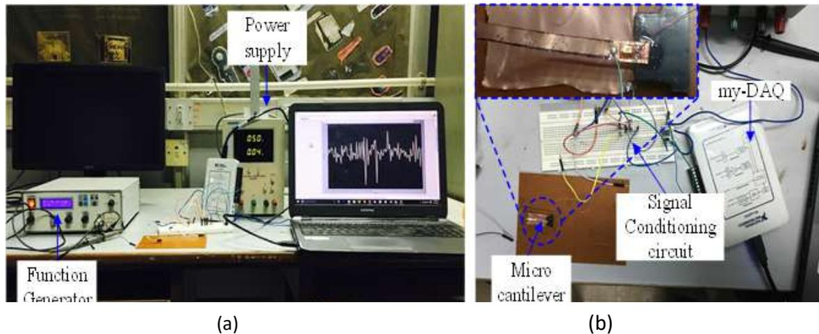
**Figure 4: (a) Experimental setup (b) Polyimide based microcantilever data acquisition circuit**
