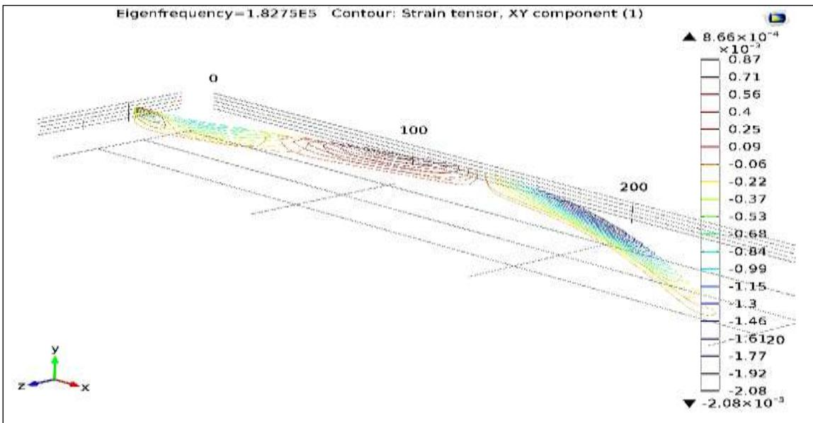
Figure 3 (b): Graph showing Corresponding strain plot on the microcantilever
