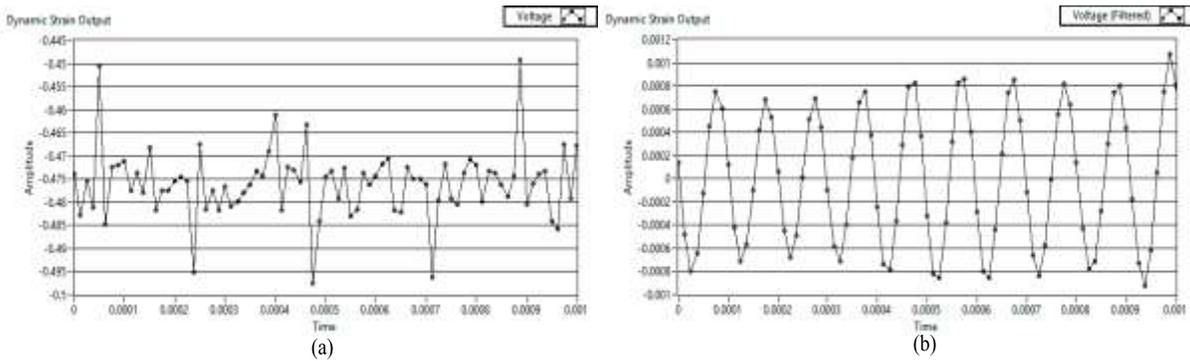
Figure 8: Dynamic strain output at time instant t2 (a) Unfiltered (b) Filtered
