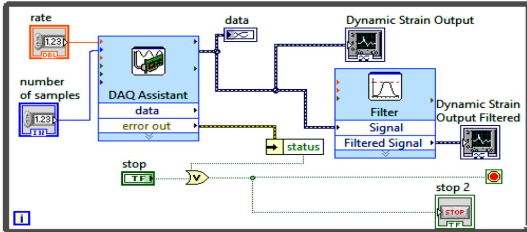
Figure 5: Block diagram of the data acquisition system on LabView
