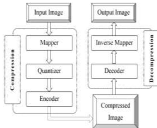
**Figure 1. Process of Image Compression and Decompression**
