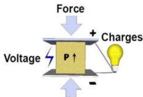
Fig,3 Working of piezoelectric material
