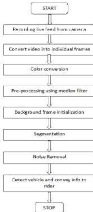
Fig. 2. Flowchart showing steps of video processing algorithm.
