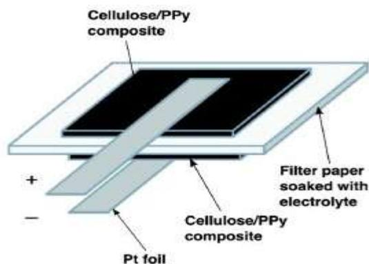
Fig 1: Paper Battery Parts
