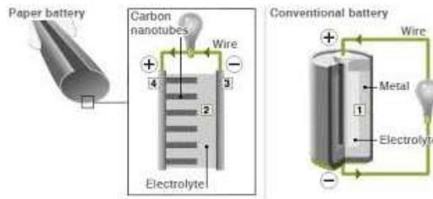
**Fig 2 : Working of Paper Batteries**
