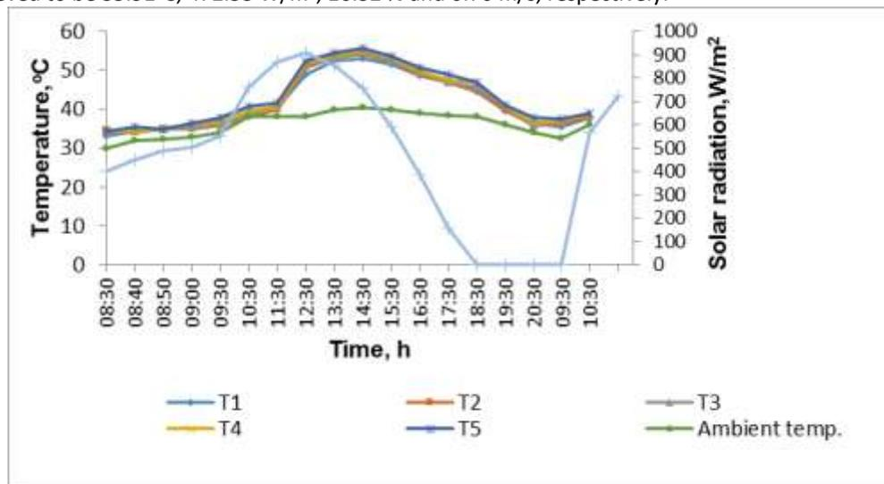
Fig. 3 Temperature variation in solar cabinet dryer
