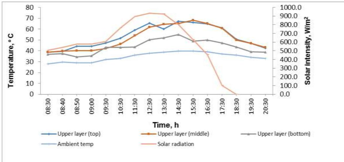
Fig. 4 Temperature developed in the heat storage system at full load condition
