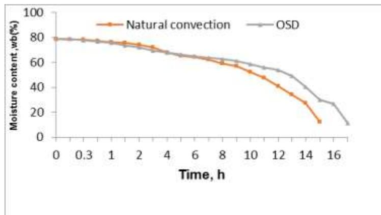
Fig. 5 Variation in moisture content of ginger slices in solar cabinet dryer and open sun drying
