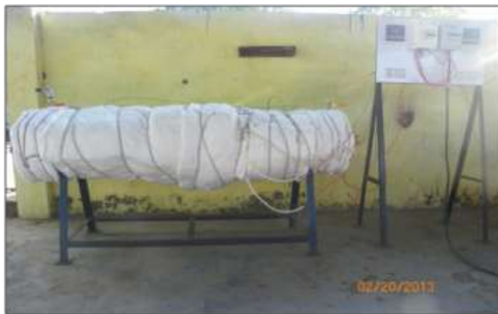
Fig.1. Experimental set-up of horizontal bio-char reactor System
