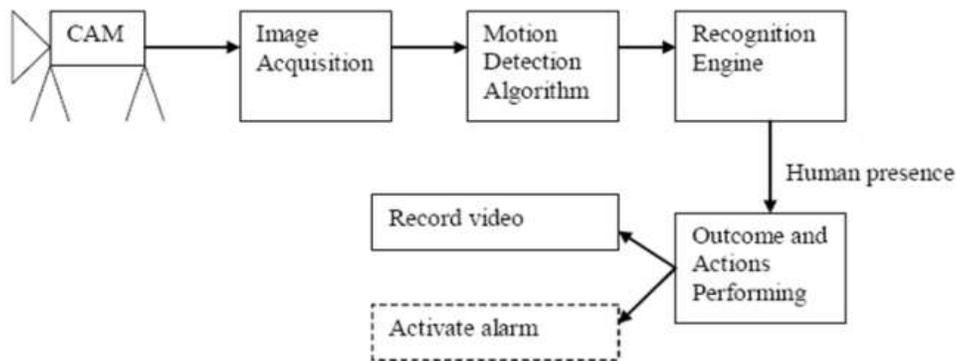
Figure 1: Overview of a basic motion detection application system
