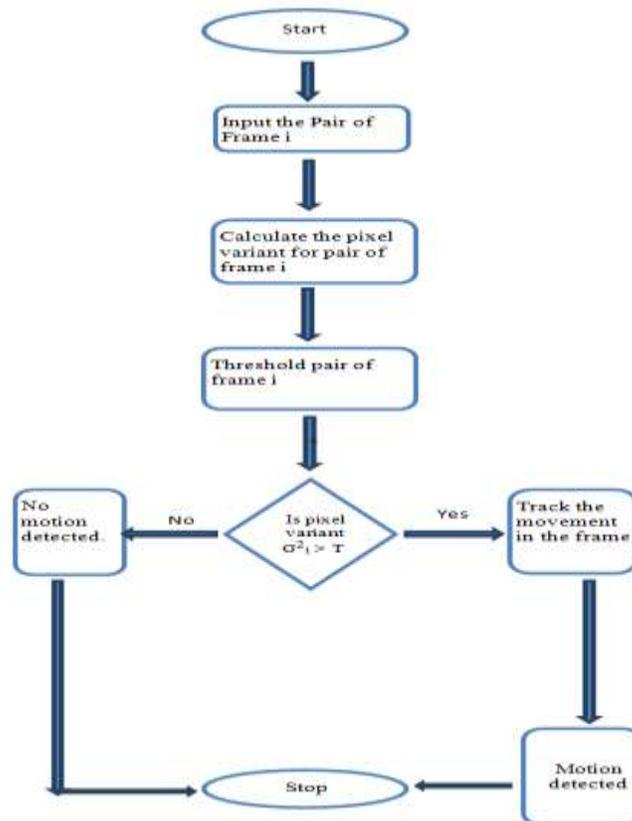
Figure 5: Flowchart of motion detection method
